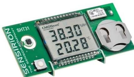
Figura 2.1 – *Data logger* (Smart Gadget Sensirion) Fonte: RS Components@. (2018)
