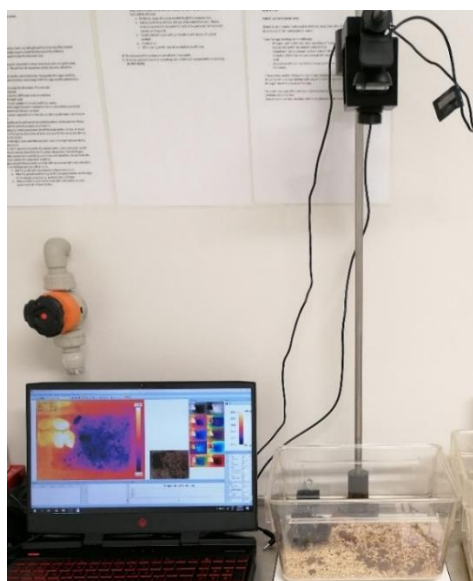
Figure 12. Equipment setup for the infrared and visible camera
