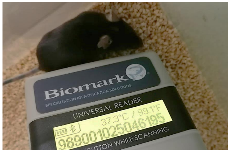
Figure 15. Subcutaneous dorsal temperature from thermosensitive PIT-tags reading.
