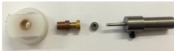
Figure 3.12. Example of the assembly of a stationary shoulder tool [41].
