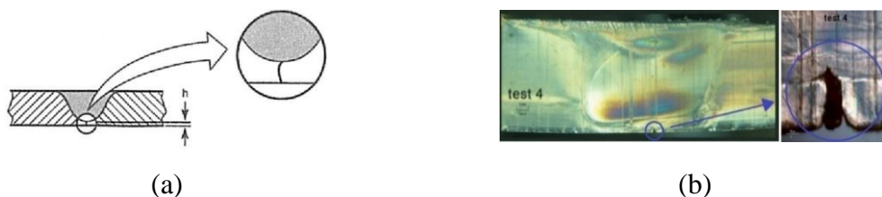
Figure 3.4. Root defect: (a) schematic illustration adapted from [28] and (b) real example [29].
