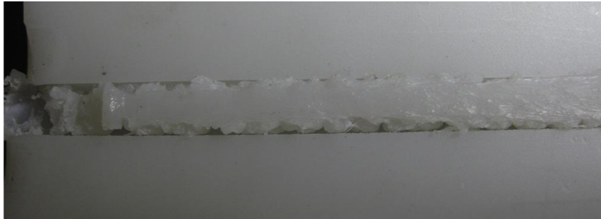
Figure 4.41. Result of welding performed with shoe temperature below 70°C, adapted from [59].
