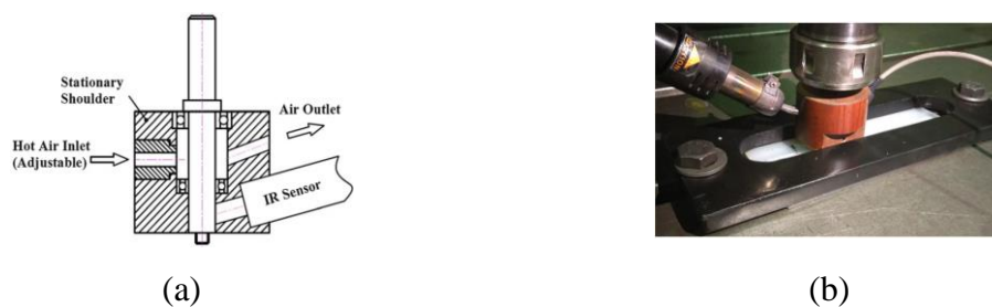
Figure 3.16. (a) Schematic illustration of the new developed tool heated by a hot air gun. (b) Welding assembly during the process [47].
