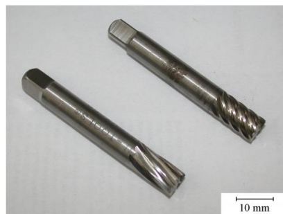
Figure 4.33. Conventional milling tools used in the FSW of PP plates [54].
