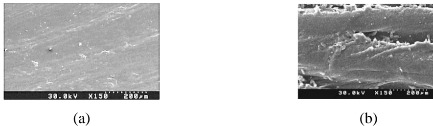
Figure 4.25. Microstructure obtained with welding speeds of: (a) 12.5 mm/min and (b) 8 mm/min [77].
