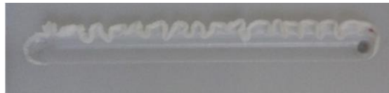
Figure 3.5. Real example of flash defect produced by FSW [30].
