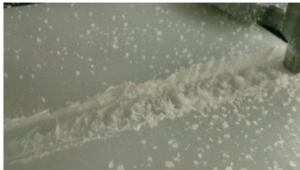
Figure 4.15. Milling effect during FSW due to the use of high welding speeds [62].
