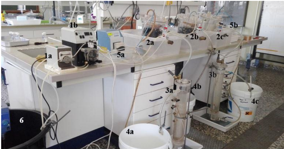
Figure 3.3: View of the experiment assembled and operating in the laboratory; 1a & 1b: peristaltic feeding pumps, 1a feeding MBBR and 1b feeding IFAS and AS; 2a: IFAS reactor; 2b: MBBR reactor; 2c: AS reactor; 3a: decanter for the IFAS reactor; 3b: decanter for AS reactor; 4a & 4b & 4c: receiver tanks for effluent from MBBR, IFAS, AS respectively; 5a & 5b: Sludge recirculation peristaltic pumps from IFAS and AS respectively; 6: feeding tank.
