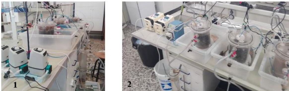
Figure 3.1: View of the initial experiment arrangement; 1: Initial arrangement with the first pumps, incubation period; 2: Second arrangement with new pumps, beginning of the experiment.
