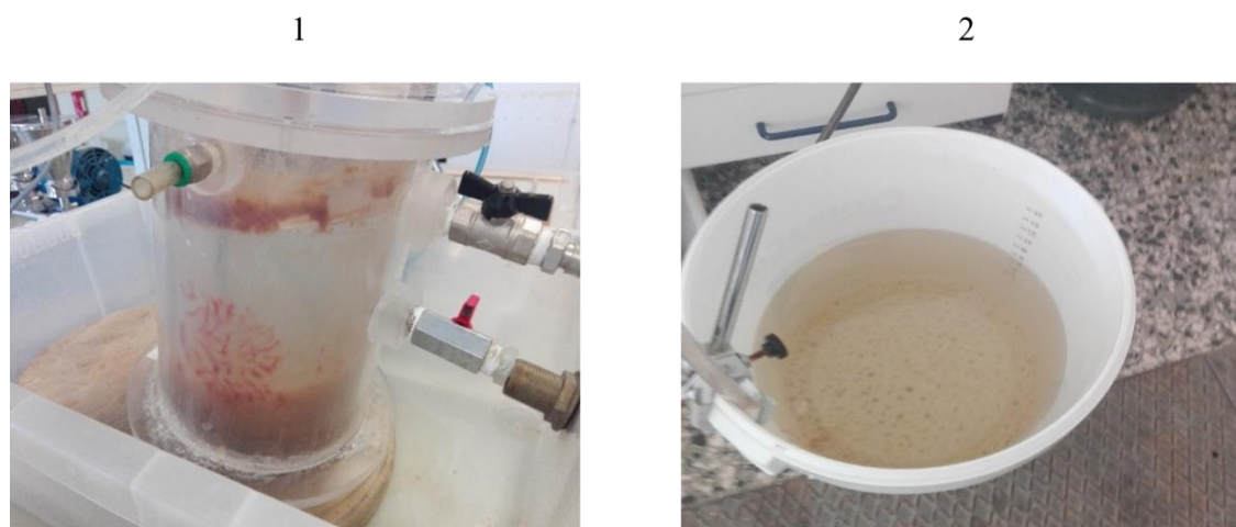
Figure 0.1: Problems observed in AS in period B: 1- Reddish sludge spots observed in the AS system in period B; 2- Reddish spots appearing in the bottom of the treated effluent tank.
