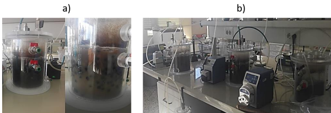
Figure 3.4: a) Inoculation of the carriers in the reactor. IFAS reactor in the left and MBBR reactor at the right. b) Initial experimental set up, corresponding to the AS sludge inoculation period and preliminary trial.
