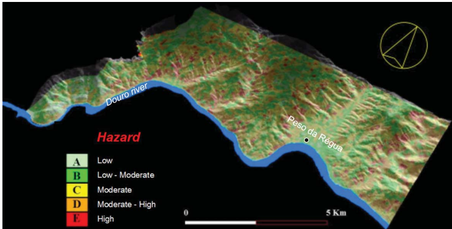
Figure 9. Landslide hazard map for the Peso da Régua region (Douro river valley).
