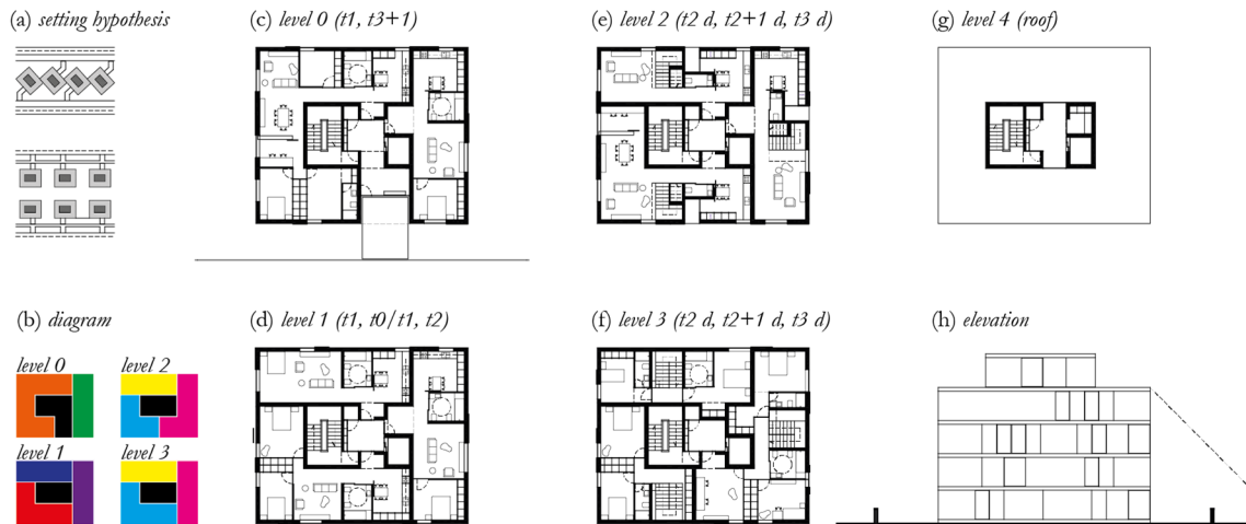
Figure 46. Illustration of a basic case of multi-story adaptation, where it was necessary to add an exception to the m:(2,3) shapes in level 0.
