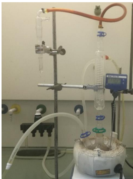
Figure 17. Experimental setup for the synthesis of SPIONs by thermal decomposition.
