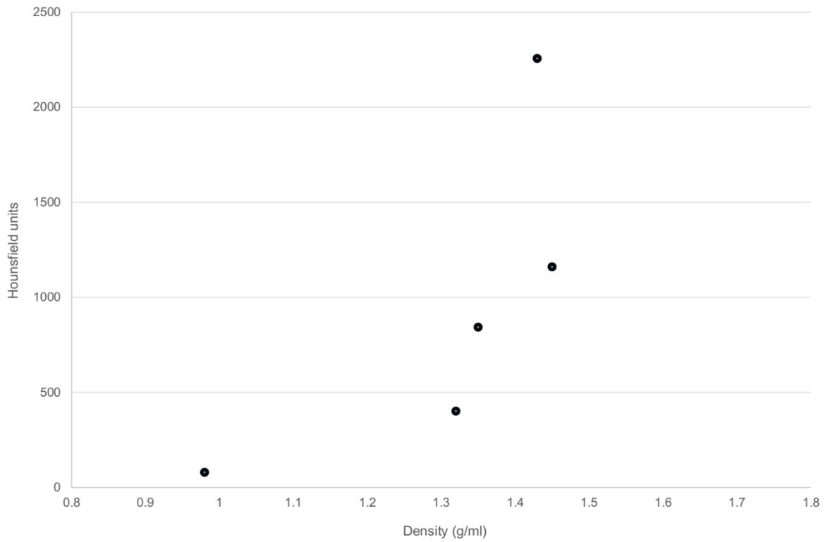
Fig. 5 – Scatter plot - relationship between the density of each block and the corresponding Hounsfield units in the CBCT image.
