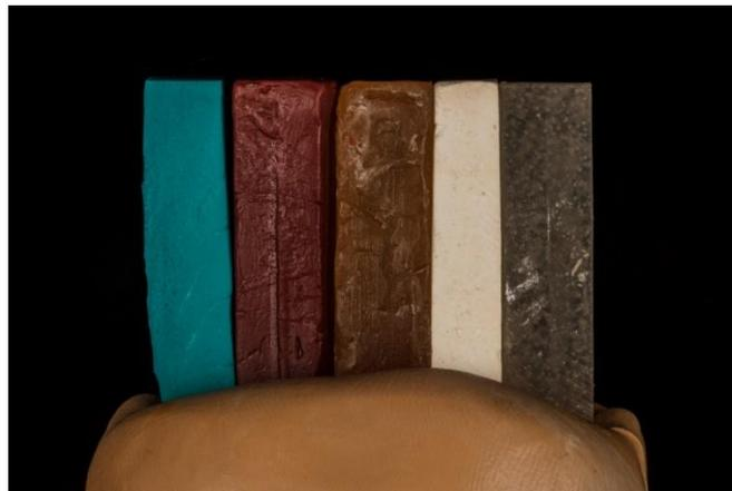
Fig. 1. Phantom materials on the mold made from Polyvinyl siloxane Impression Material (From right to left: Acrylic, Plaster ISO-type III, Join Wax, Impression Compound Color Red and Polyvinyl siloxane Impression Material)
