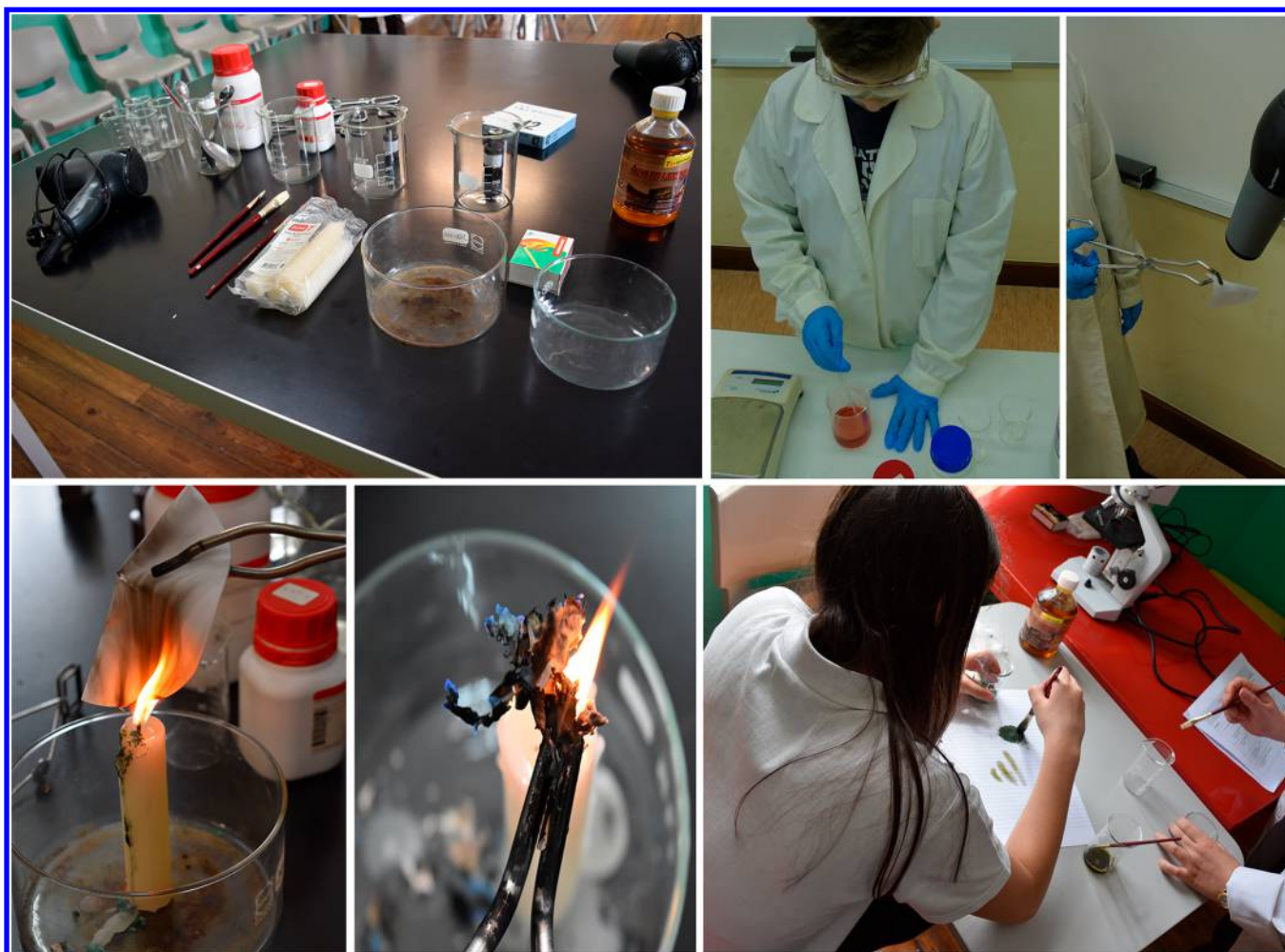
Figure 3. Photos taken during an informal session at a middle school (students aged 12–14). From left to right: materials needed, student preparing one of the solutions, students drying the soaked filter paper with a hair drier, student burning the filter paper using a candle, blue ashes, and student using the just made green pigment mixed with linseed oil.
