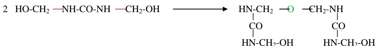
Equation 2 Creation of ether linkage
