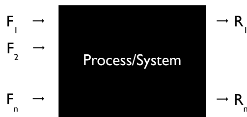
Figure 5. The blackbox view of a process or system, where the factors, F , control the response, R . Usually, n \gg m .
