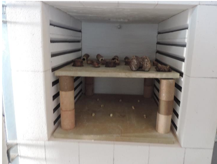
Figure 2.5 – Muffle furnace, Barracha, K-3 three-phased, 14A, containing teeth (bottom) and some sectioned bones (top).
