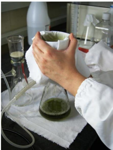
Figure 2.14 Hot filtration of one of the samples performed under suction: cotton filtration followed by filtration in a silica filter.
