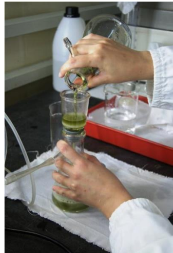
Figure 2.14 Hot filtration of one of the samples performed under suction: cotton filtration followed by filtration in a silica filter.
