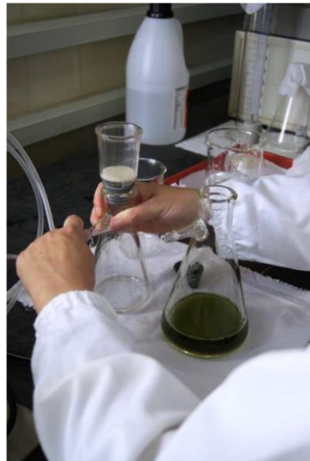
Figure 2.14 Hot filtration of one of the samples performed under suction: cotton filtration followed by filtration in a silica filter.
