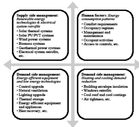
Figure 3 Main categories of building retrofit technologies (Ma Z. et al., 2012).
