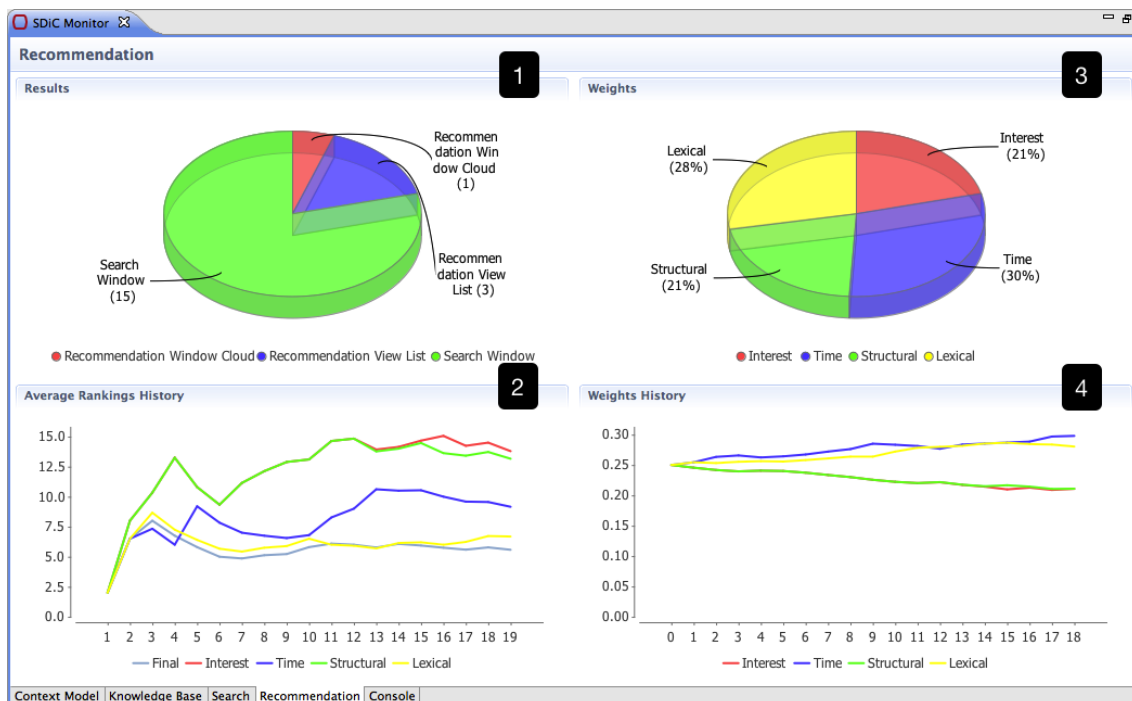
Figure 4.9: A screenshot of the monitor interface showing information about the context-based recommendation, including the number of selected recommendations (1), the distribution of the recommendation weights (2), the evolution of the average rankings of selected recommendations (3), and the evolution of the recommendation weights (4).
