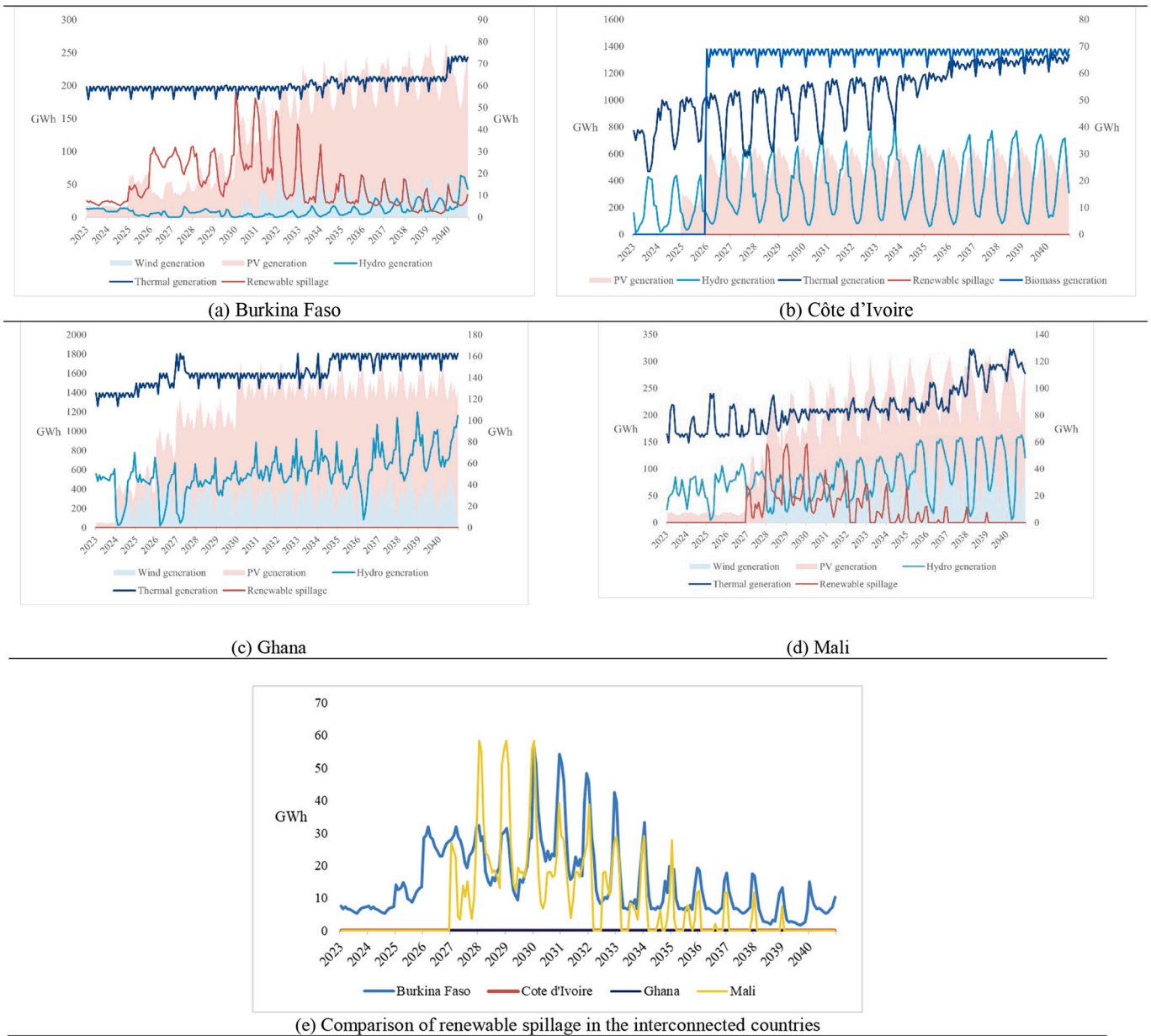
Fig. 8. Electricity generation by source (GWh) and generation spillage (GWh) in the interconnected countries between 2023 and 2040 for the base-case scenario (left axis for thermal and hydropower generation; right axis for renewable generation and spillage).
