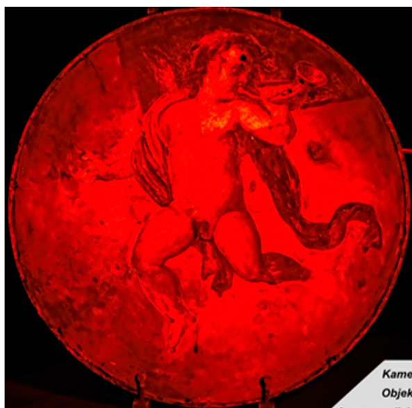
Figure 6. IR-Picture depth analysis with a camera (4000 K); objective filter (OG 590 nm yellow-red); excitation light (500-500 nm green) (Fig.: LKA Hannover).
