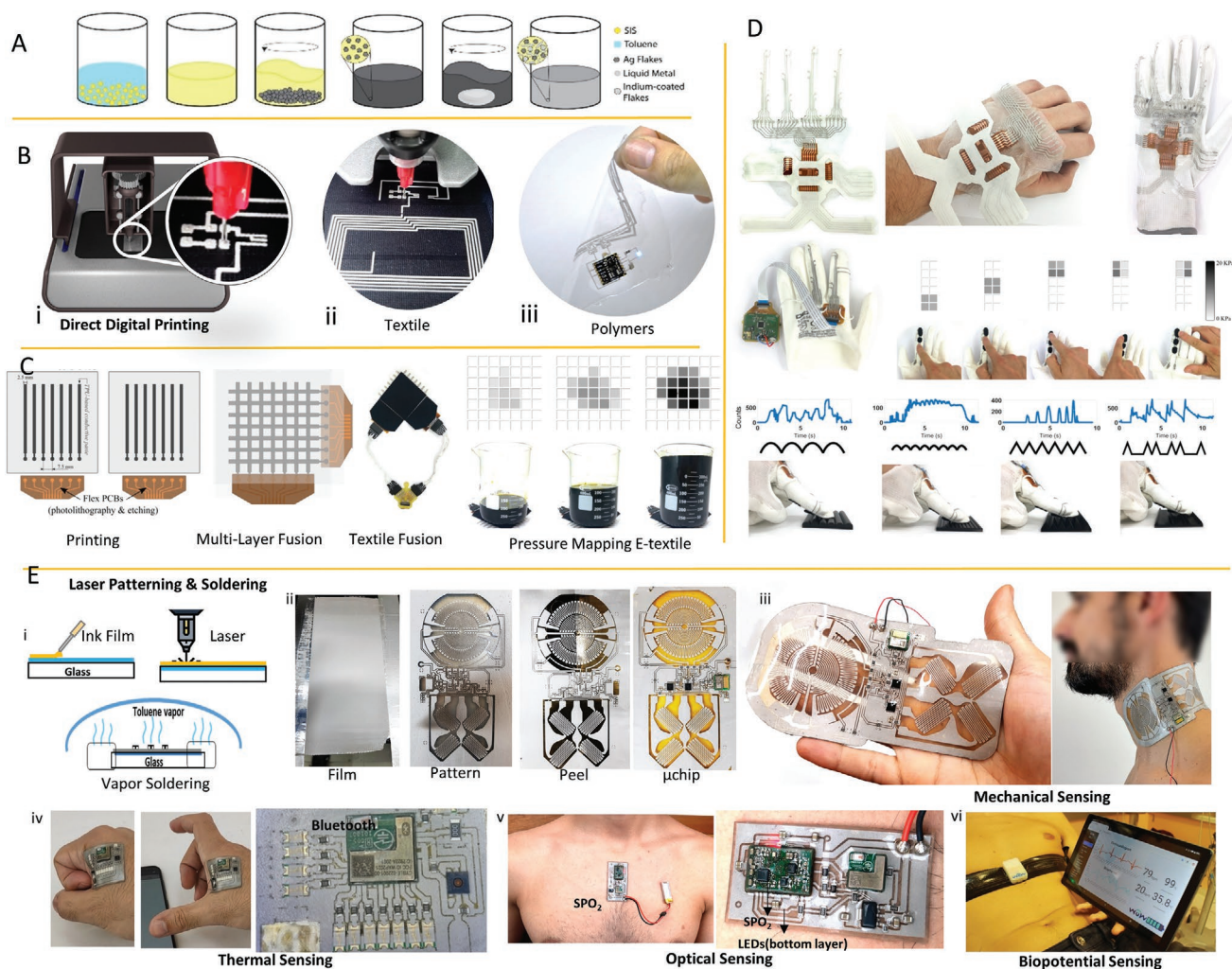
Figure 2. A) Synthesis of sinter-free stretchable biphasic ink. B) Digital Printing of e-patch and e-textile circuits C) Example of a pressure mapping e-textile fabricated through digital printing. D) Example of a wearable glove with printed bending and pressure sensors, its application in pressure sensing, and surface texture classification. E) High-resolution Laser Patterning of the circuits using an accessible IR laser and Single-step vapor-assisted soldering of miniaturized components: i) Example of the fabrication steps. ii) No solder material or thermal treatment is necessary. Examples of chip-integrated soft-matter epidermal biostickers for mechano-sensing iii), thermal iv), optical v), and electrical sensing vi). These patches can be used for monitoring respiration and physical activities iii), body temperature iv), heart rate, and SPO 2 v). The belt presented in E-iv measures ECG, heart rate, respiration, temperature, and body motions simultaneously.
