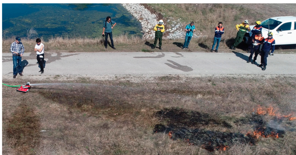
Figure 11. Initial experiments on the field with the pan and tilt nozzle unit directing the water jet to the fire area, based on the fire sensor information.
